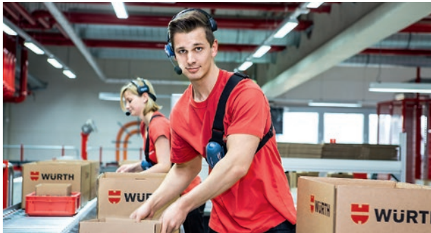
Pick-by-voice: The new Würth logistics center West uses a pick-by-voice system. Orders are wirelessly transmitted to the picker by the inventory management system.
